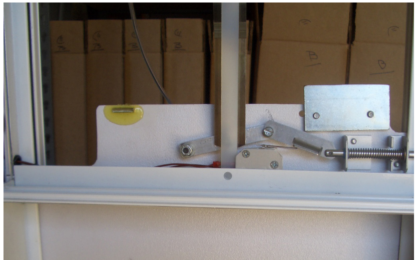
View of back of pet door showing lock and micro switch
